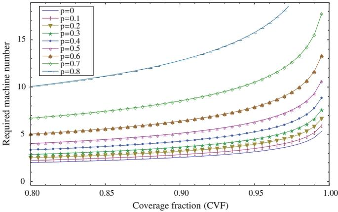
**Fig. 9** Required machine number by PPP versus coverage fraction under different failure probability  $p$ . The numbers have been normalized by the required number of ideal non-overlapping deployment under zero failure probability
