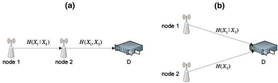
**Fig. 4** The two cases of compress-and-forward transmission with its corresponding transmission flow. **a** Serial transmission. **b** Parallel transmission
