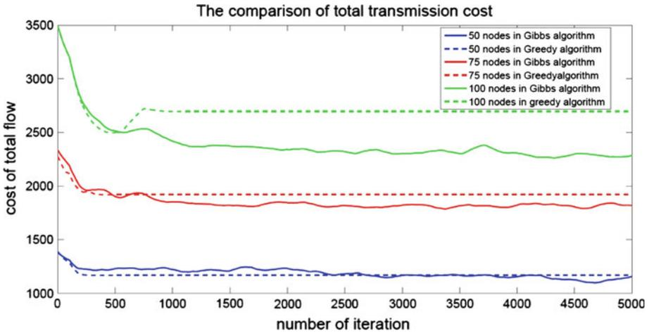
Fig. 7 The simulation result of Gibbs algorithm compared with greedy algorithm
