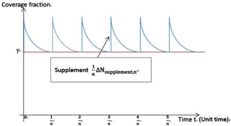
**Fig. 11** The  $\gamma$  is the coverage fraction level we want to maintain all the time, so we supplement machines by the number  $\frac{1}{n} \Delta N_n$  per  $\frac{1}{n}$  unit time
