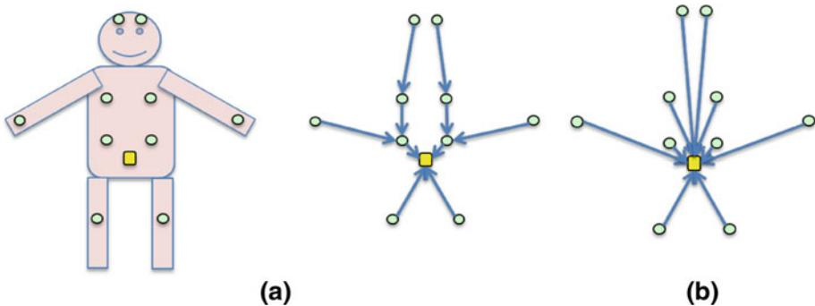
Fig. 3 a To hop or b not to hop for sensors with a robot. a Multi-hop ad hoc networking (from sensors to data aggregator). b One-hop star networking (from sensors to daa aggregator)
