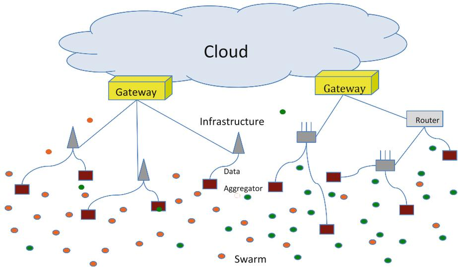
**Fig. 1** Cloud-based M2M communications
