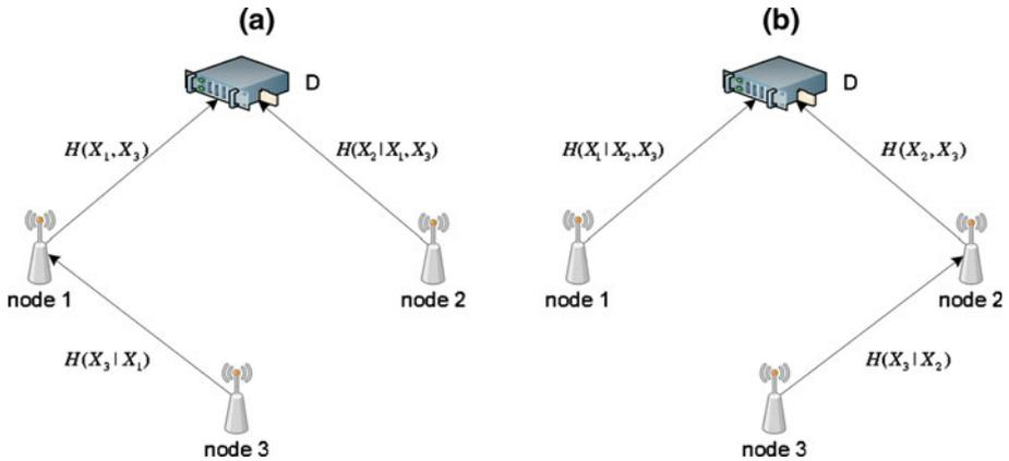
**Fig. 5** In case **a** and **b** with different forwarder of node 3, the total transmission will be different. **a** Node 3 choose node 1 to be forwarder, and node 2 can overhear the two transmission flows. **b** Node 3 choose node 2 to be forwarder, and node 1 can overhear the two transmission flows
