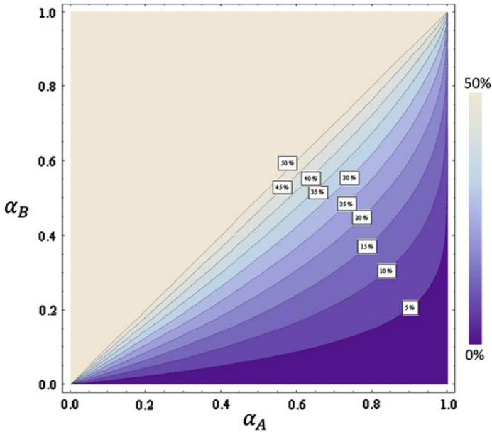
**Fig. 12** The percentage of reduced sensors for operator *A* under cooperation with operator *B* by using Shapley value, where  $\alpha$  is the coverage requirement
