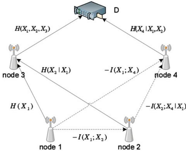
Fig. 6 With adding of compensation flow, the flow conservation rule is satisfied
